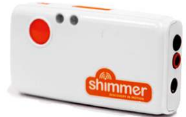
Shimmer3 GSR sensor, the primary sensor used for this study
